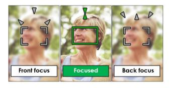
The innovative UI applies Dual Pixel CMOS AF phase-difference detection AF technology to also tell the user if the focus position is in the front or the back. An useful feature when shooting in 4K, which requires strict focus accuracy
