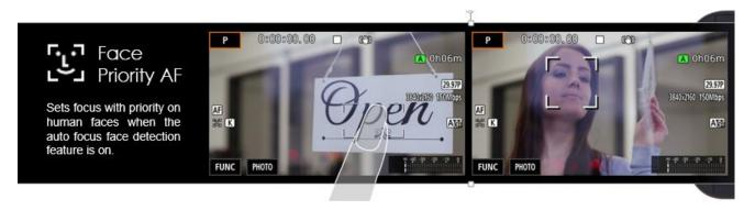
The touch panel enables smooth, intuitive operation of Dual Pixel CMOS AF. When used in combination with the face detection AF, users have the flexibility to choose the right auto focus shooting solution they need.
