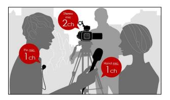
The on-board 4ch audio independent settings let users set recording levels, input sensitivity, and limiters for each channel
