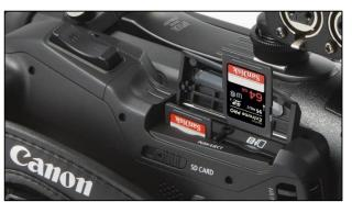
Relay and simultaneous recording are provided via Dual SD card slots, which helps to expand recording times and to create an immediate backup.
